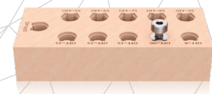
The Stump Die 3D master file will allow to check printer resolution enabling to choose the relevant OFF value into ModelPro aiding to achieve a proper fitting.
